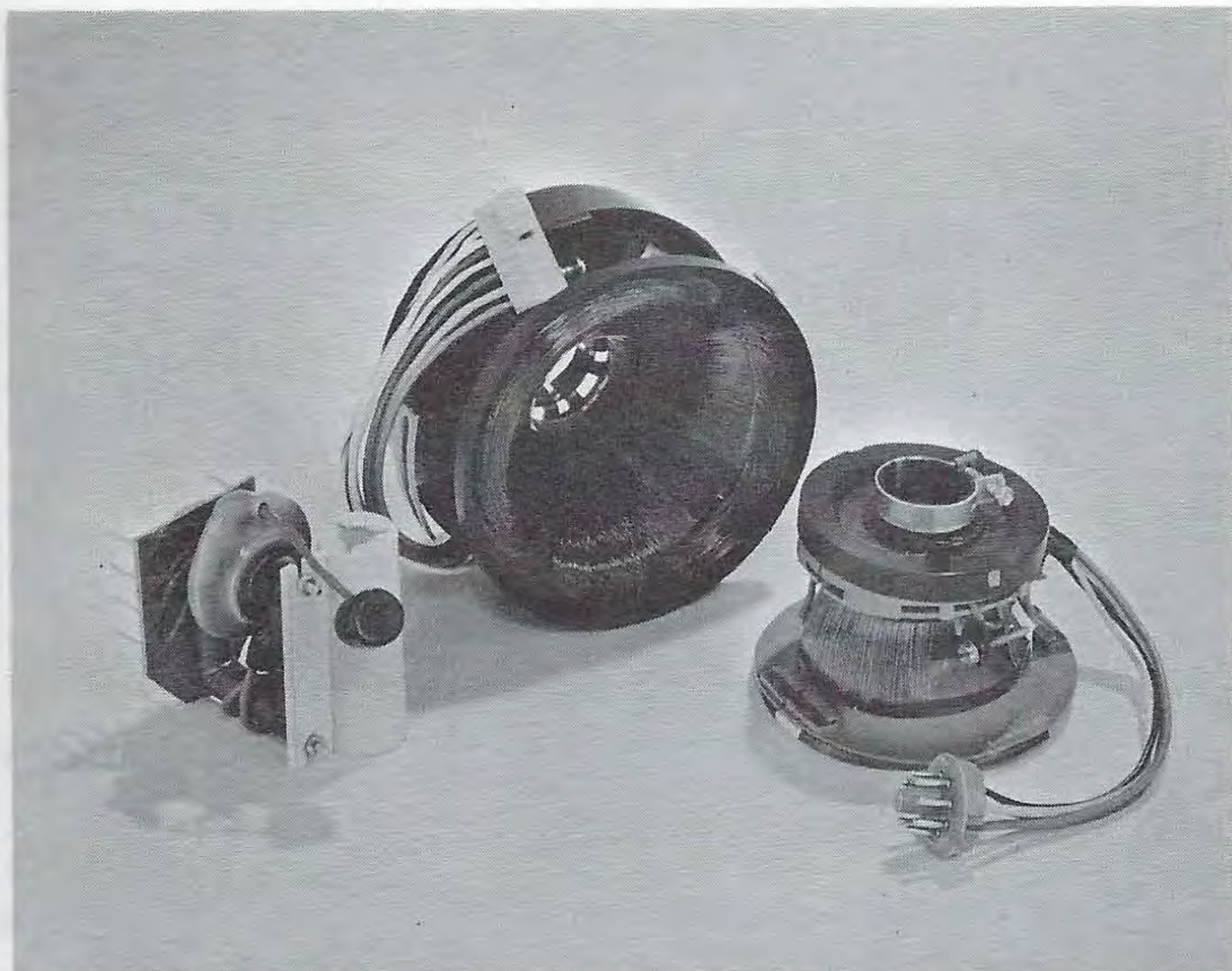
"Mini-Yoke" (center) for leading color television receivers. Special "fly-back" transformer and deflection yoke with vertical toroidal winding for high resolution video display use.
