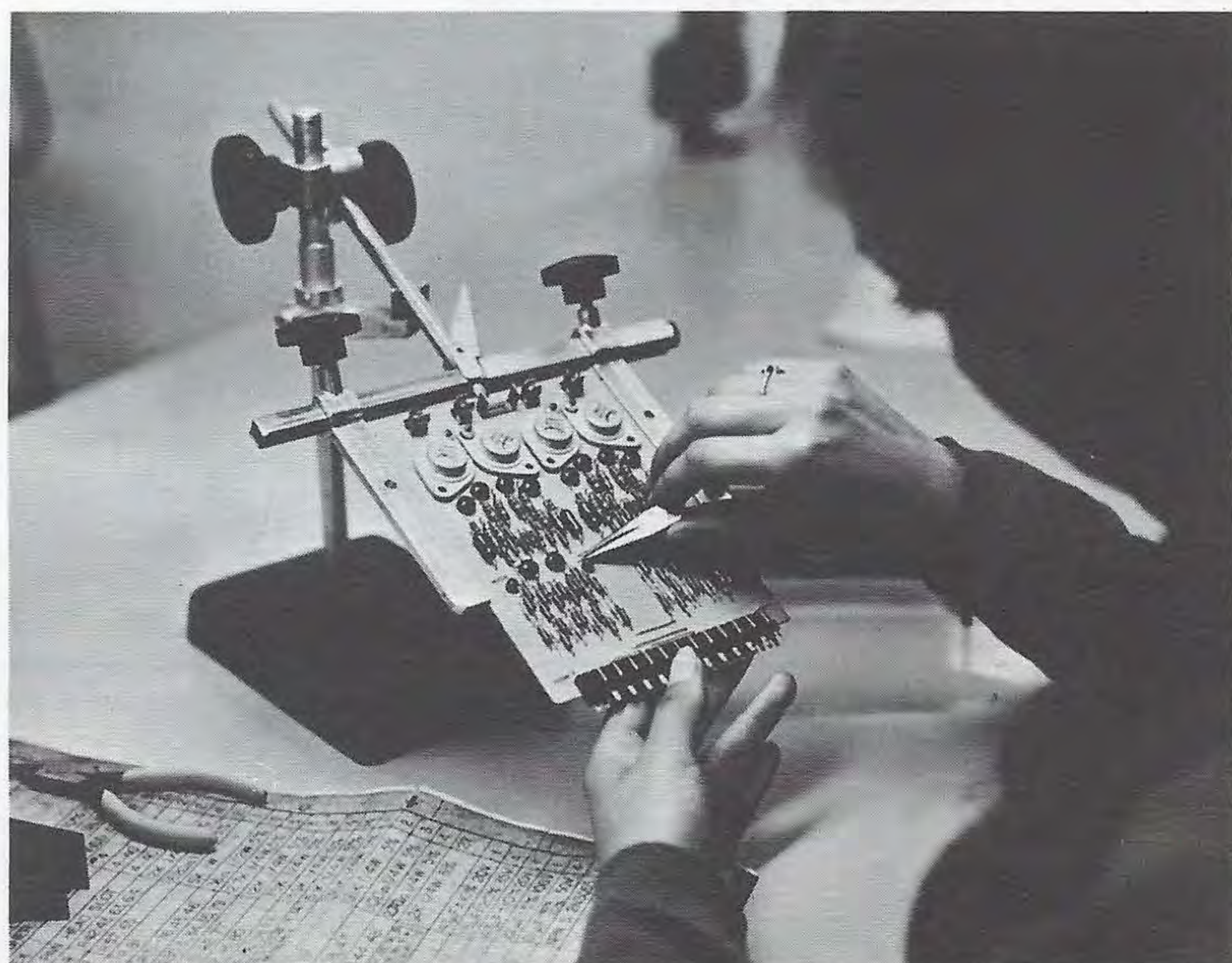
Loading components on printed circuit card preparatory to wave soldering.
